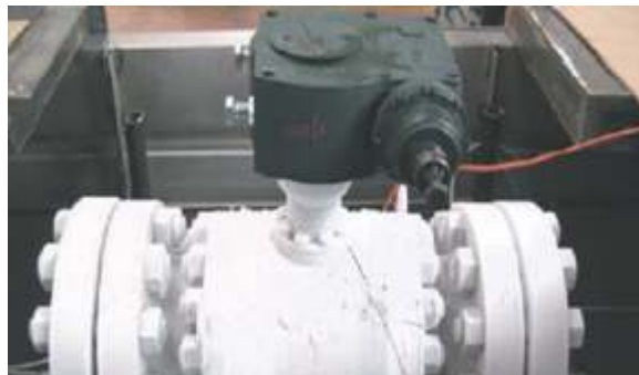
Ball valve cryogenic test
