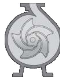
Expanding Volute Casing (Standard Pump)
